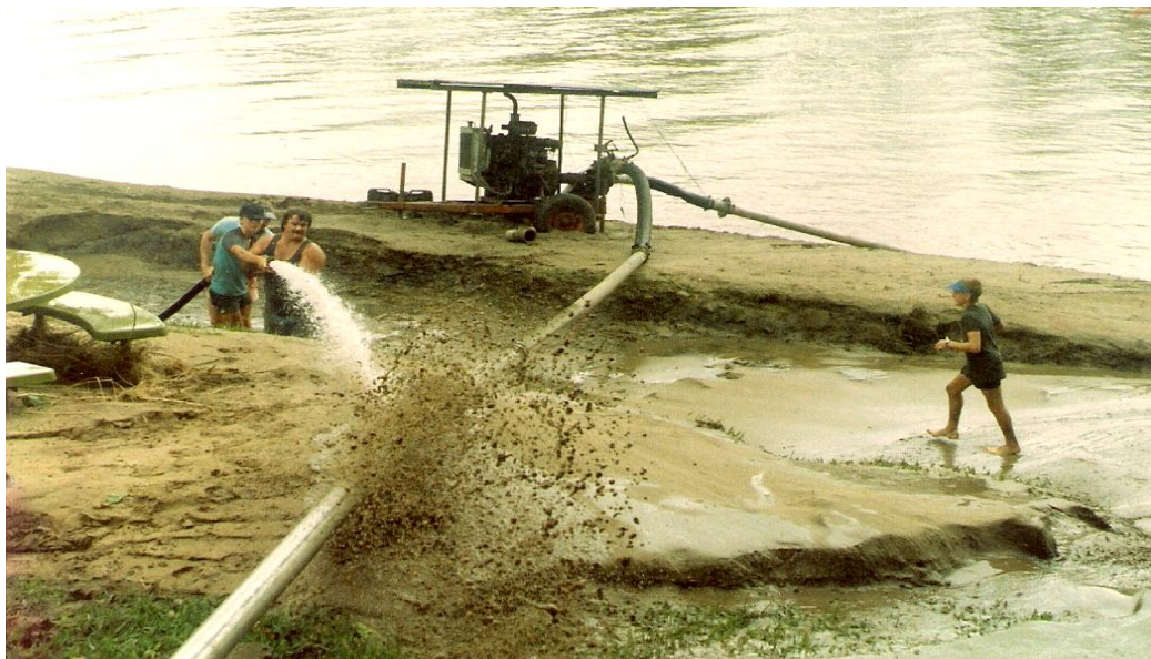
A pump borrowed from local farmer to wash away deep silt left by a flood.
